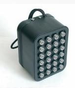
A1220 MONOLITH consists of electronic unit with a screen and a keyboard and a 24 element matrix antenna array, working on the principle of double-crystal transducer. The antenna array elements are spring-loaded, which allows to test uneven surfaces.
